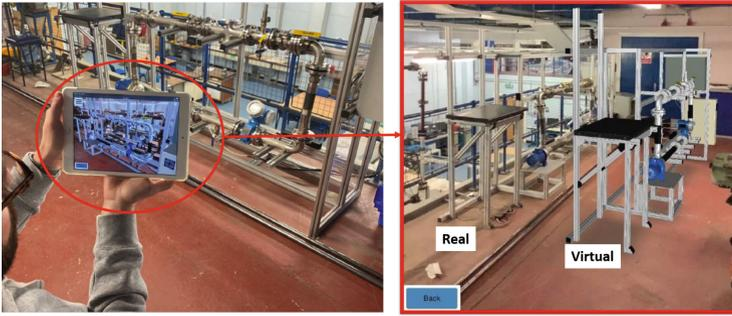
**Fig. 1.** It shows the real oil plant with its virtual model placed side-by-side.
