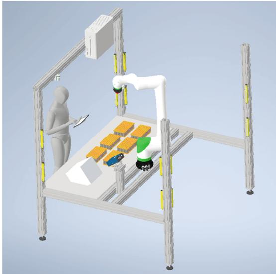
**Fig. 2.** DemoDatenPro demonstrator: A collaborative robot assists the disassembly of a product. Additional information can be augmented with an projector. Several sensors are collecting disassembly information.
