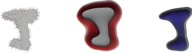
**Fig. 3.** Piecewise polynomial SDF of the `035_power_drill` object from the YCB dataset [6]. The ground truth mesh with 700 non-uniformly distributed training samples is shown on the left. The center and right image show the reconstructed mesh and level sets (positive in red and negative in blue).
