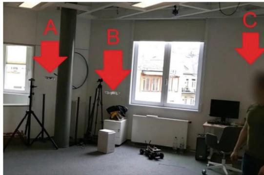
**Fig. 3.** Augmented Reality test with CrazyFlie 2.1 and OptiTrack Prime indoor motion tracking system mounted on the ceiling, where “A” marks the real drone, “B” the pre-played digital twin of the drone and “C” is the human observer.
