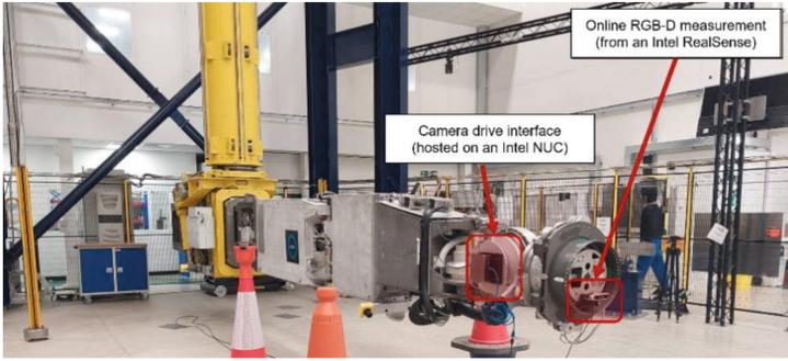
Fig. 2. Experimental setup with an RGB-D camera integrated with TARM [13].
