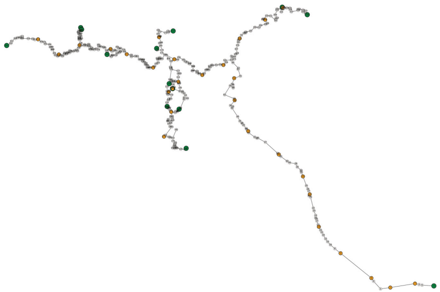
Fig. 9 Sole-Mare-Vento network: yellow nodes represent the location of the CSs, green nodes are the endpoints of the paths. The longest stretch is the trail arc from Termoli to Ortona, with a length of 62.4 km. The origins or destinations of the paths are Torino, Rozzano, Vieste, Trieste, Assago, Verona, Fiesole, Samone, Piacenza, San Giorgio di Nogaro, Albareto, Rivalta sul Mincio, Marzabotto, Greve in Chianti
