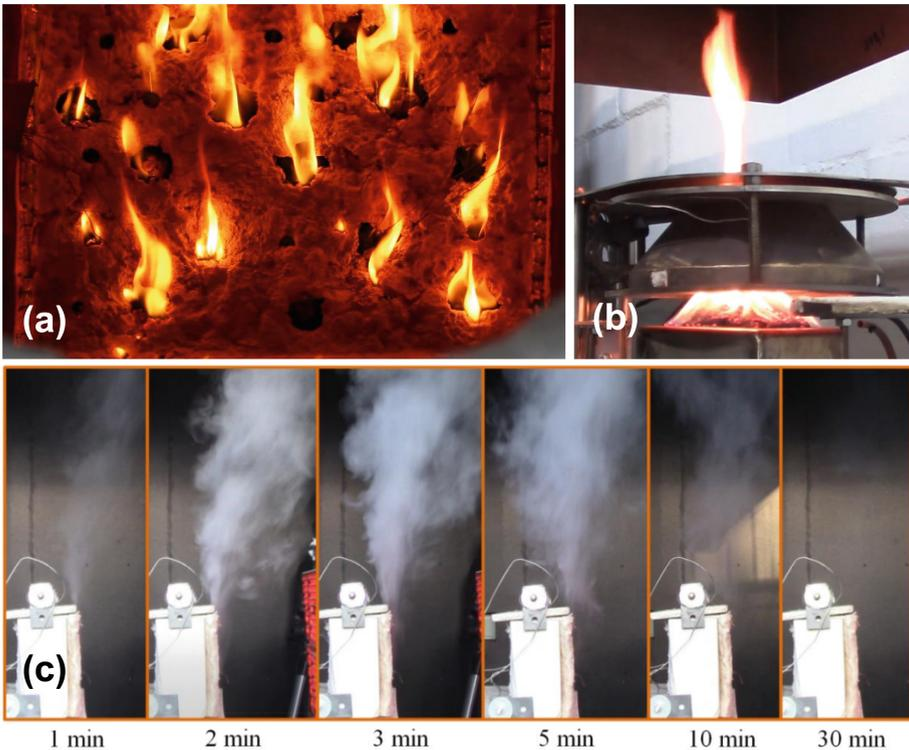
**Fig. 1.** Consideration of fire behaviour showing (a) flaming ecobricks within a wall after standard furnace testing [5] (each flame occurs in front of an ecobrick), (b) ignition of biomass under a cone calorimeter [18], and (c) smoke emissions from a bricks incorporating RESIN8 [19].
