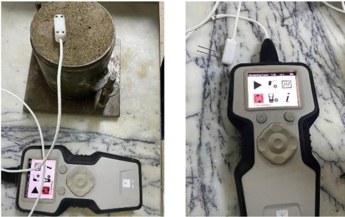
Fig. 2. The thermal conductivity measuring equipment
