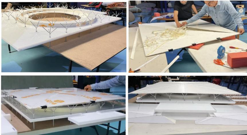
**Fig. 3.** Construction of the rigid model.
