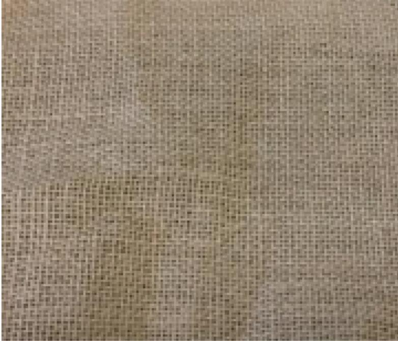
**Fig. 2.** Coir geotextiles used as a reinforcement in the study
