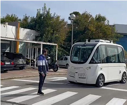
**Fig. 5.** Experiment 2: the pedestrian is crossing on the crosswalks and the shuttle bus stops.
