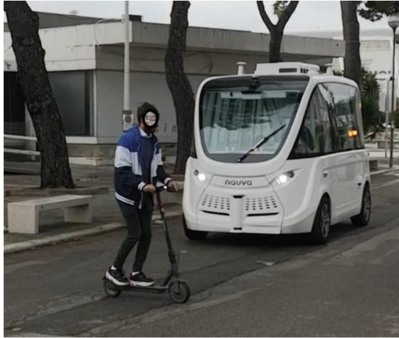
**Fig. 7.** Experiment 5: E-scooter crosses the road in front of the shuttle bus, in an unexpected way.
