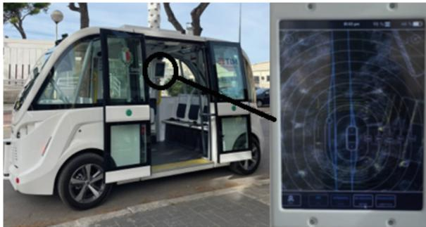
**Fig. 3.** Automated shuttle by Navya (external view) and focus on the desktop showing how the shuttle perceives the external environment through its sensors (in blue the predetermined route, in yellow the detected obstacles as point clouds).
