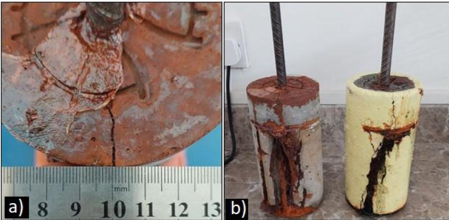
**Fig. 4.** a) Crack width measurements, b) CC and CC-SC specimens after corrosion
