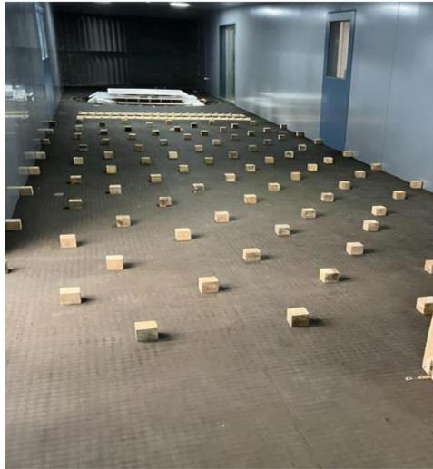
**Fig. 4.** Roughness elements in the test section of the wind tunnel.
