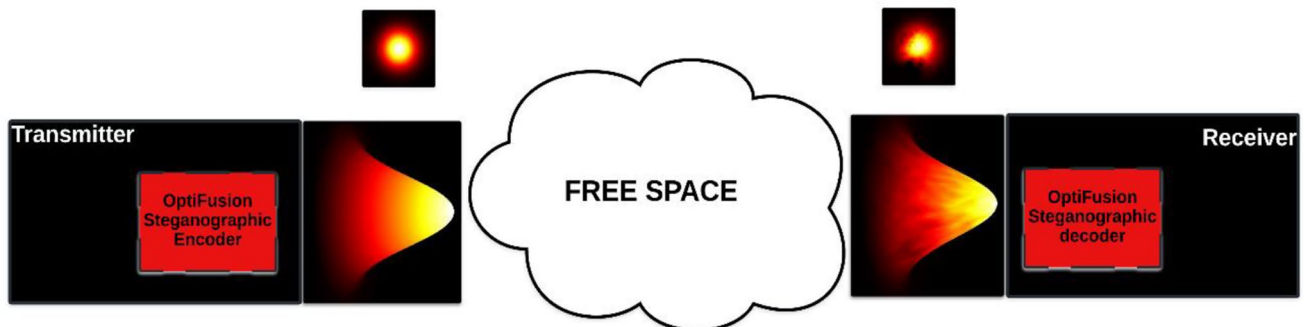
Fig. 5 Overview of propagation of a Gaussian beam in free space, based on the OptiFusion Steganography method, with the effects of turbulence
