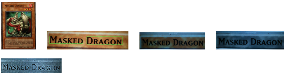
Fig. 3. These images are our preprocessing steps-the sequence takes. From left to right, we show that the first image is the CCG card we capture, the second is the detected words, the third is the denoised name, the fourth is the grayscaled image, and the final image is the threshold image.
